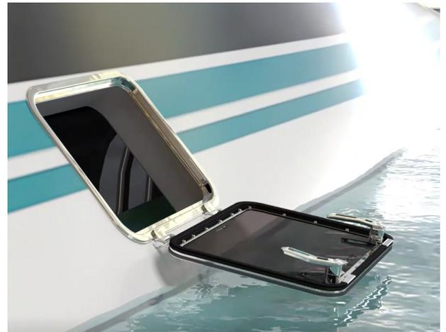
Swedish manufacturer Rutgerson Marin has now taken on the challenge by developing an escape hatch where the acrylic lens is bolted to the frame rather than glued. To reduce the risk of leakage ever further, Rutgerson's escape hatch has double seals and an innovative flush frame in stainless steel which gives minimal resistance in the water and significantly reduces the pressure on the hatch.
